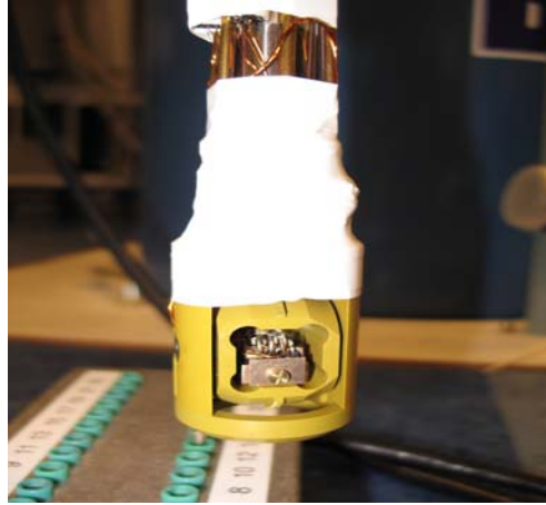
Figure 7.6 Sample holder with sample mounted inside the cup of the Swedish rotator. This cup can be rotated 270 degrees with respect to the initial position shown here. This can be done with a resolution of 0.2 degree.
